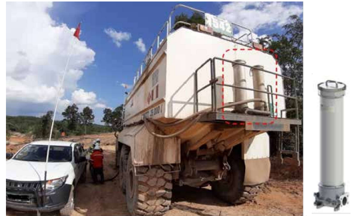
Instalasi filter Hydac di Fuel Truck
